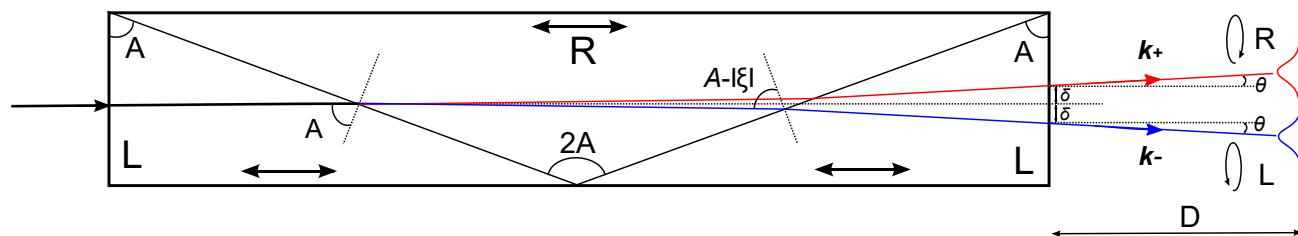
With metasurfaces in which the sign of the geometric phase depends on the polarization
