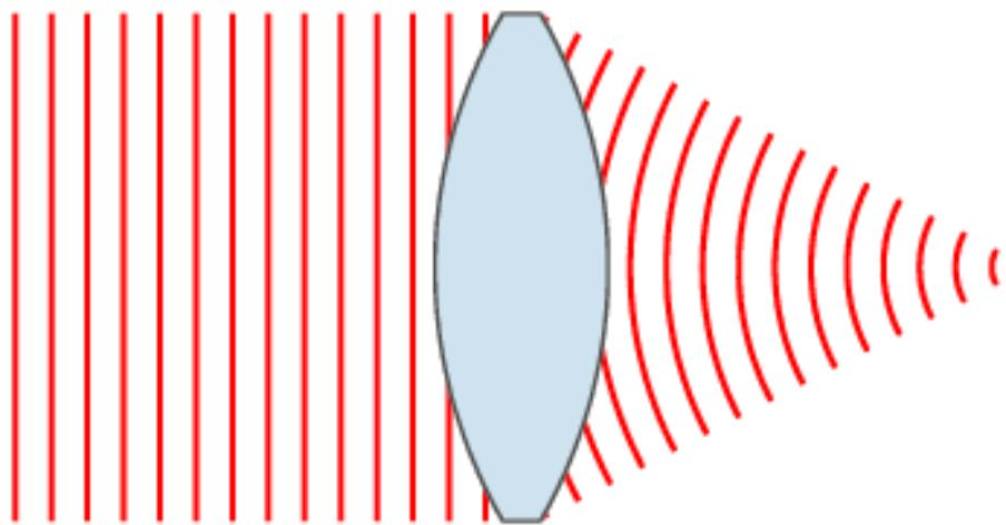
As the wave hits the lens, it is the centre of the wave that meets the glass first and so this part of the wave is slowed down first. The outer portions of the wave 'catch up' so increasing the curvature to form a converging beam
