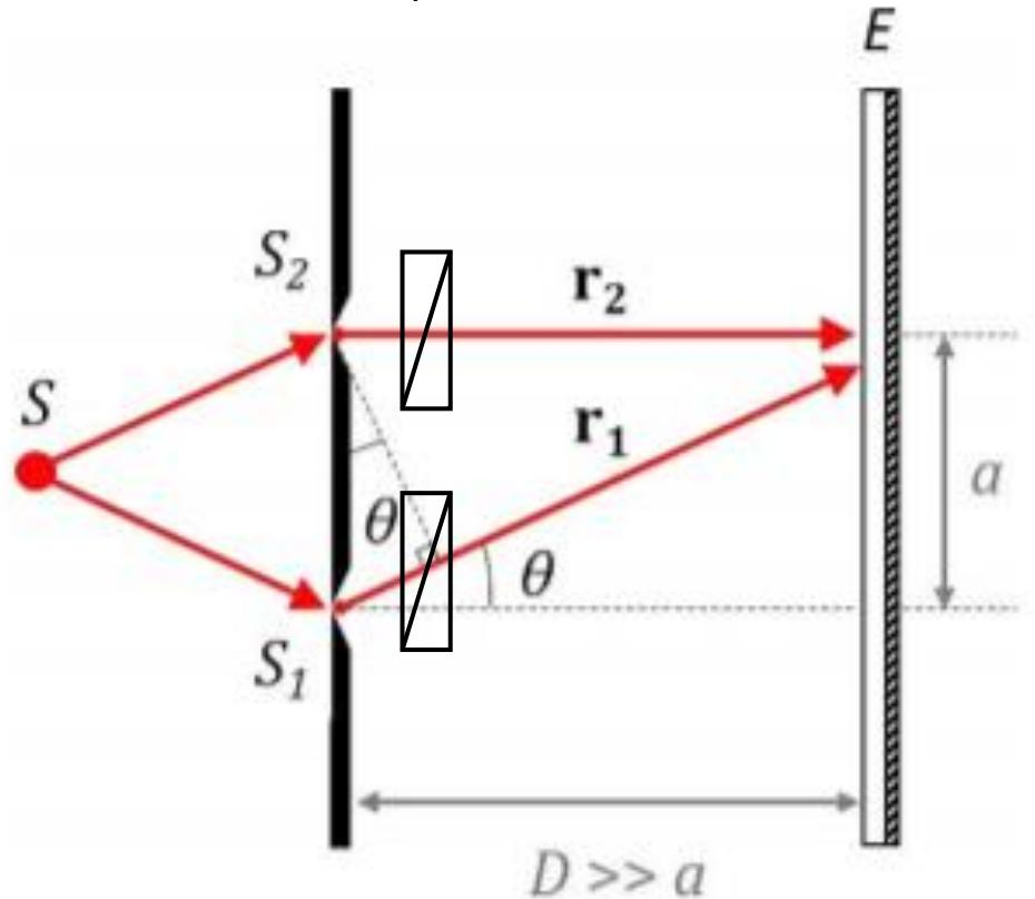
Calcite experiment (split in H and V components)
