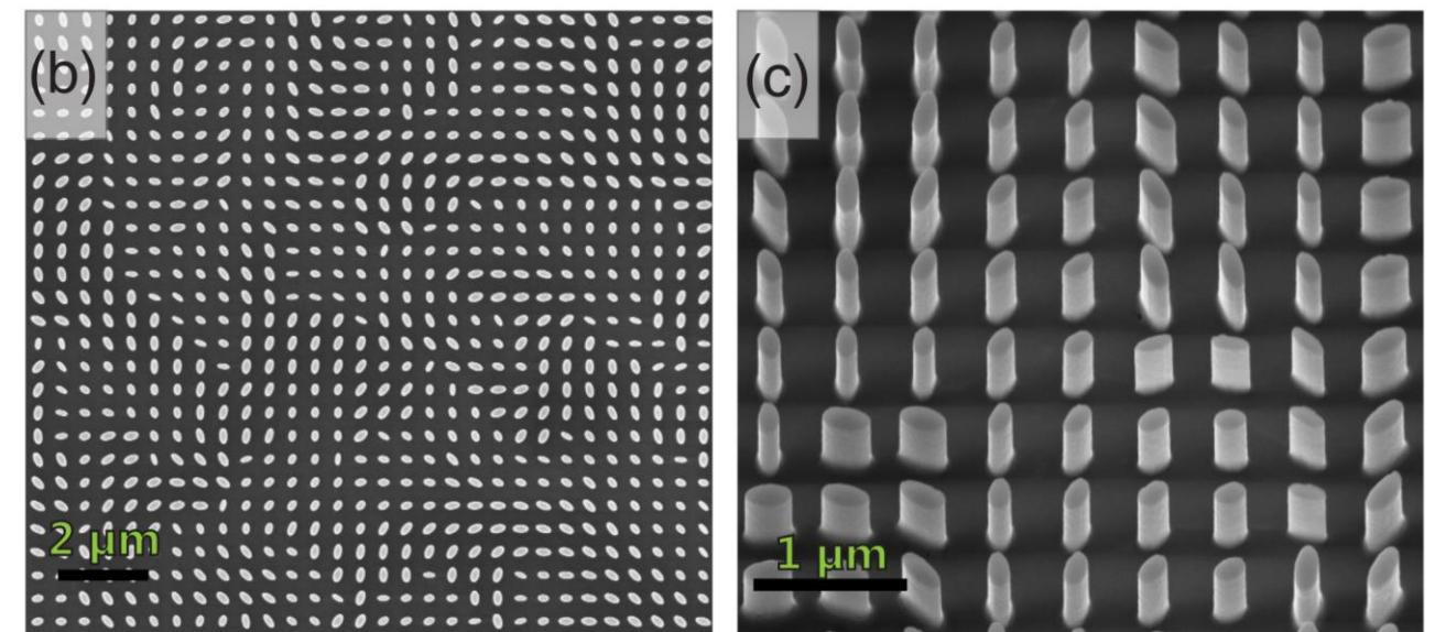
Metasurface with  $\text{TiO}_2$  Pillars with shape anisotropy
