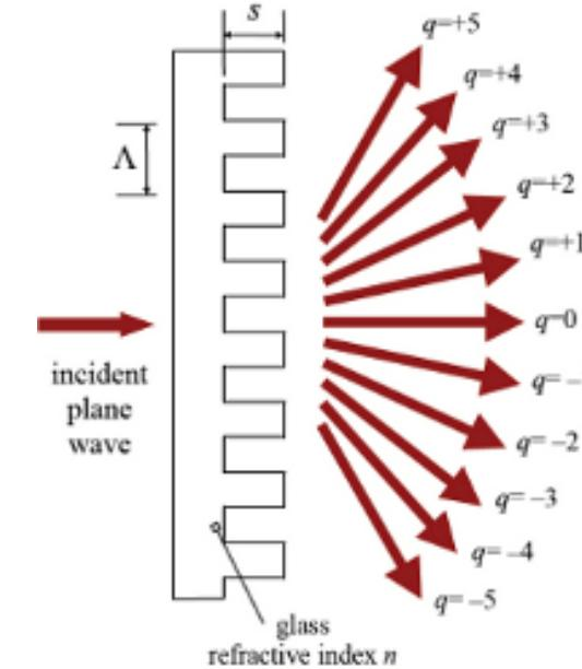
A transmission grating is a periodical structure with steps (binary here) that diffracts light
